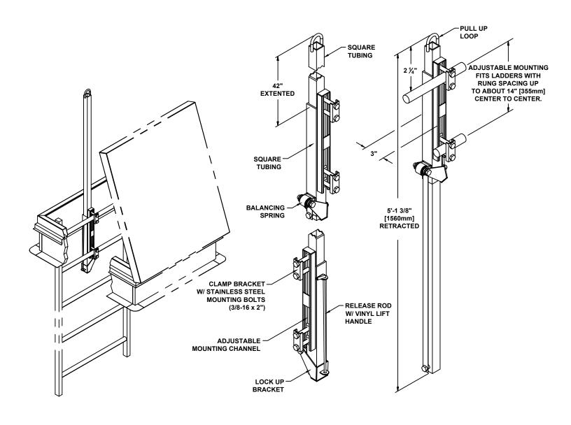
CLAMP BRACKET MAY BE REVERSED TO ACCOMMODATE RUNG SIZES OF 3/4" TO 1 1/4" WITH STANDARD 2" BOLTS FURNISHED. LARGER RUNGS WILL REQUIRE LONGER BOLTS.
